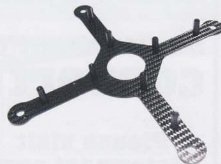
The chassis is cleanly cut from 1 mm carbon fibre plate. Note the pillars to hold the upper chassis parts
