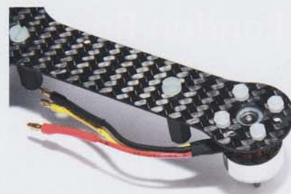
Note the nylon bolts holding the motors – in a crash, they'll break rather than the chassis
