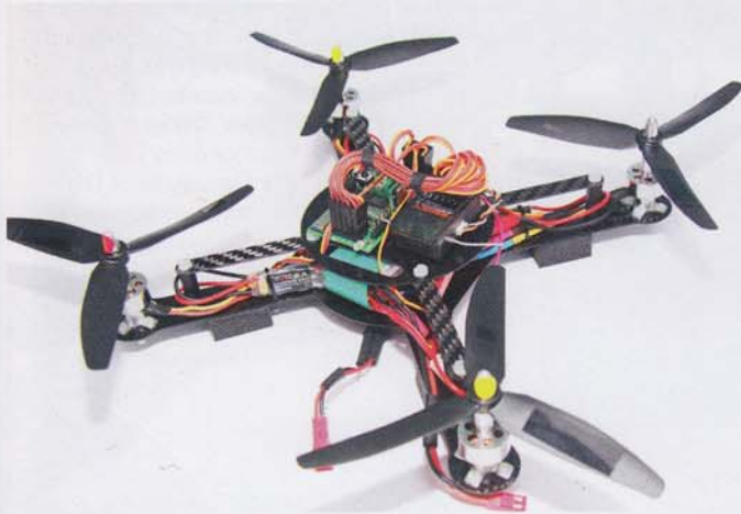
The QuadPod pretty much built in an evening, just awaiting the clear dome top
