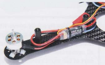
I changed the layout of the ESC wiring slightly, wrapping it around the pillars to keep it neat
