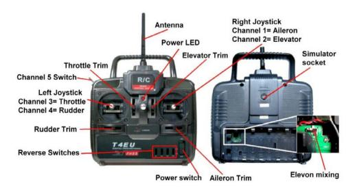
**Aileron Control (CH1):** When the aileron stick is moved to the right, the right aileron is raised and the left one lowered, and the aircraft rolls to the right. When the aileron stick is moved to the left, the ailerons move in the opposite directions and the aircraft rolls to the left.
